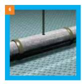
After weighing the amount of Isocynate and Polyol according to given ratio, stir thoroughly and pour into the drilled hole.
