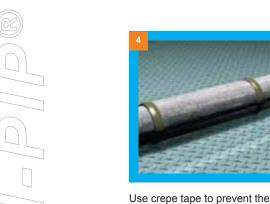
Use crepe tape to prevent the foam leaking out from the edge of the sheet.
