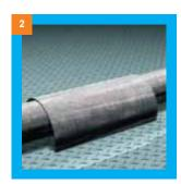
Place the galvanized iron sheet on top of the cladding.
