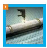
Drill a hole at the centre of the galvanized iron sheet for pouring PU chemicals inside.
