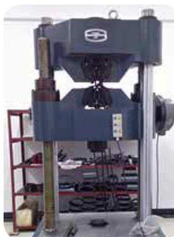
Tensile Strength Testing Machine
