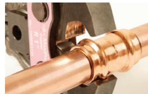
9. Align jaws squarely on the fitting
